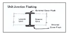
Allow 3mm - 5mm clearance around louvre perimeters. Maximum louvres widths not to exceed 1500mm for single modules unless additional support is provided.
